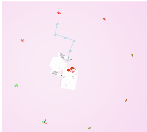
Fig. 1: A top view of an example motion generated by a mobile manipulator to perceive and grasp a target object. The target object is highlighted in the red box. The circle around the scene shows the candidate viewing angles, and green and red correspond to more informative and less informative viewing angles. The light blue line shows the actual viewing trajectory followed by the robot.
