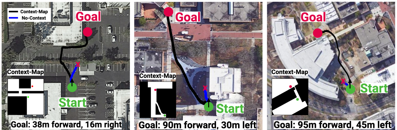
Fig. 4: We test our policies in 3 novel environments in the real-world. The routes contain many obstacles including bushes, buildings, cars and pedestrians that the robot has never seen during training. The Context-Map policies (black) are able to navigate hundreds of meters to reach the goal 100% of the time. In comparison, the No-Context policies (blue) beeline towards the goal, resulting in episode failures.
