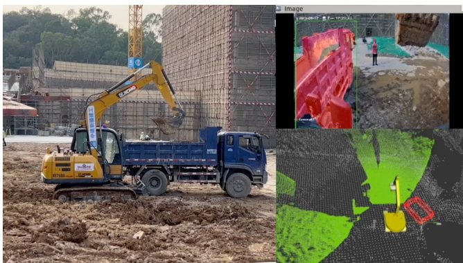
Fig. 5: Autonomous truck loading. During the operation, the 3D truck pose is estimated as shown in the upper-right window, and the task area is designated as a red box as shown in the lower-right window.
